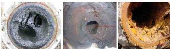
The same problems from paraffin and or asphaltene deposits happen in the pipeline increasing pressure and damaging pumps and even blocking pipelines with costly consequences in lost production, maintenance and equipment replacement.
